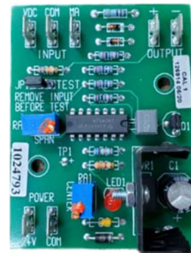
Drives up to 4 controllers per Input Board with Pulsed 24VDC, 1 Second time base
