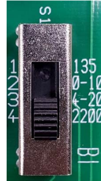
Example switch setting at 2200 ohm
