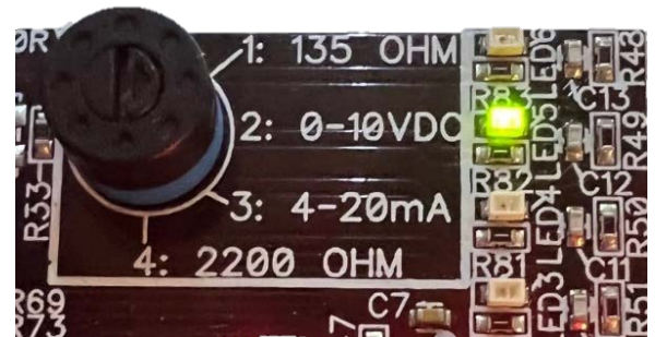
Example switch setting at 0-10VDC
