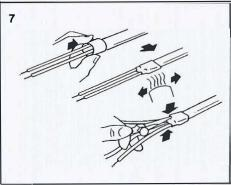
Slide the 1/2" x 11/2" heat-shrink tube over the bus wires and partially over the inner jacket. Heat shrink the tube; while still hot, pinch the center of the heat- shrink tube between the bus wires with needle-nose pliers.
