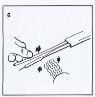
Slide the  $^{1/8}$ " x  $5^{1/2}$ " heat-shrink tubes on the bus wires. Shrink the tubes with heat gun or soft flame torch.
