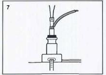
Make sure the sealing grommet is set in the base.
