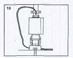
Mount junction box with non-threaded opening for <sup>3</sup>/<sub>4</sub>" conduit, using the sealing gasket and lock ring to hold in place, or use a junction box with a <sup>3</sup>/<sub>4</sub>" inside threaded hub. Ground the braid pigtail to conduit with a clamp (not provided).
