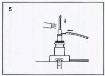
Slide the black ¹/e" x 5¹/2" heat-shrink tubes on the bus wires, and the green/ yellow ¹/4" x 5¹/2" heat-shrink tube on the ground pigtail. Heat shrink, using a heat gun, or soft flame torch, moving the heat source back and forth.
