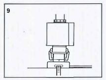
Mount junction box with non-threaded opening for <sup>3</sup>/<sub>4</sub>" conduit, using the sealing gasket and lock ring to hold in place, or use a junction box with a <sup>3</sup>/<sub>4</sub>" inside threaded hub.
