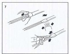
Slide the ½" x 1½" heat-shrink tube over the bus wires and partially over the inner jacket. Heat shrink the tube; while still hot, pinch the center of the heat- shrink tube between the bus wires with needle-nose pliers.
