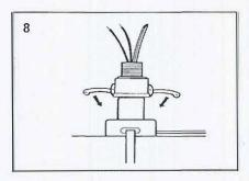
Slide the top in place and push and lock the cam levers into position. Lock cam levers by inserting the stainless steel tie wire through the holes in the ends of the cam levers and twisting together.
