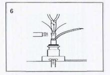
Slide the white ½" x 1½" heat-shrink tube in place over the bus wires and onto the inner jacket. Heat shrink in place. After removing the heat source, and while still hot, pinch the center of the heat-shrink tube between the bus wires with needlenose pliers.
