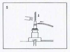
Slide the black <sup>1</sup>/<sub>6</sub>" x 5<sup>1</sup>/<sub>2</sub>" heat-shrink tubes on the bus wires, and the green/ yellow <sup>1</sup>/<sub>4</sub>" x 5<sup>1</sup>/<sub>2</sub>" heat- shrink tube on the ground pigtail. Heat shrink, using a heat gun, or soft flame torch, moving the heat source back and forth.
