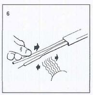
Slide the '/e" x 5'/z" heat-shrink tubes on the bus wires. Shrink the tubes with heat gun or soft flame torch.
