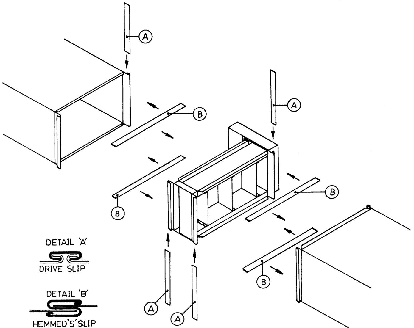
THIS HEATER HAS BEEN CONSTRUCTED FOR ATTACHMENT DIRECTLY TO THE DUCT WORK USING SLIP-AND-DRIVE CLIPS, AS SHOWN IN THE ABOVE DRAWING.
