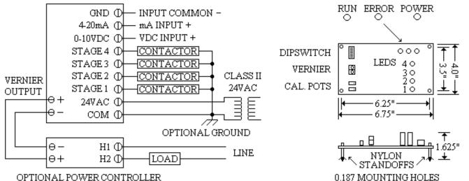
Note: GND and COM are electrically connected on the circuit board.
