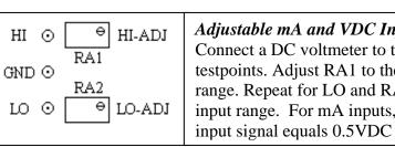
Adjustable mA and VDC Inputs (-1943): Connect a DC voltmeter to the HI and GND testpoints. Adjust RA1 to the upper input range. Repeat for LO and RA2 for the lower input range. For mA inputs, each 1mA of input signal equals 0.5VDC at the testpoint.
