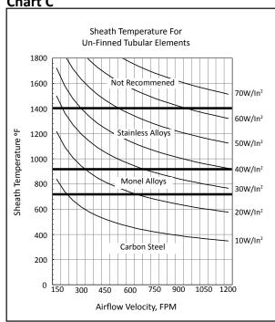
Watt Density and Sheath Materials – Table III has sheath materials recommended for each fluid and temperature. Where a range of watt densities are shown, the lower end of the range represents a more conservative design.
