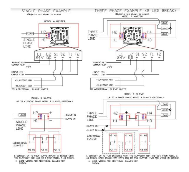
**NOTE:** All 103 Series Model A (Master) have L2 and T2 electrically connected on the input board.
