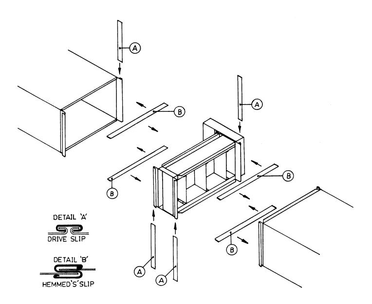
THIS HEATER HAS BEEN CONSTRUCTED FOR ATTACHMENT DIRECTLY TO THE DUCT WORK USING SLIP-AND-DRIVE CLIPS, AS SHOWN IN THE ABOVE DRAWING.
