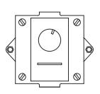
Part Number 1007002 Single stage on-off control Class I, Division 1, Groups C&D Class II, Division 1, Groups E,F,G NEMA 7 Type – SPDT 22 amps at 125-277-volts Range – 50-90°F (10-32°C) CSA Certified and UL listed
