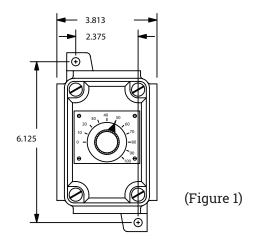
Wall mounting room set point adjuster (Figure 1) part number 810-102655 and duct mounting temperature sensor (Figure 2) part number 810-108449. Class I, Division 1, Groups C&D Class II, Division 2, Groups E,F,G NEMA type 7,9 (adjuster), NEMA type 4,7,9 (sensor) Proportional 2,200 ohm thermistor control for SCR and step controlled explosion-proof heaters Range - 0-100°F
