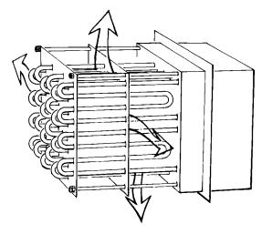
Horizontally Mounted Tubular Or Finned Tubular Heater
