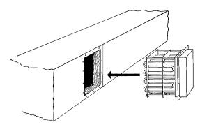
Installation Of Heater Rated For 400° F And Higher
