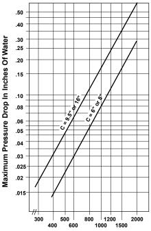
Chart B Velocity in SFPM Finned Tubular Design
