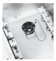
For automatic control of outlet air temperature. Adjustable over a range of 60-250° F. Outlet temperature will be lower than set point as the thermostat senses heat from elements as well as outlet air. Do not use where outlet air temperature will exceed 150° F. May also be used as an automatic high temperature thermal cutout.
