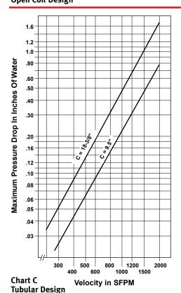
based on the airflow being parallel to the heater C dimension. For tubular design only, consult factory for pressure drop when airflow is parallel to the H dimension.
