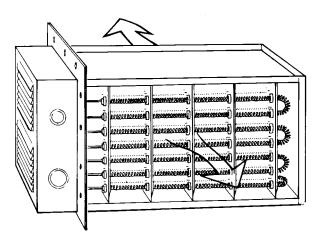
Open Coil Heater Mounted For Horizontal Airflow
