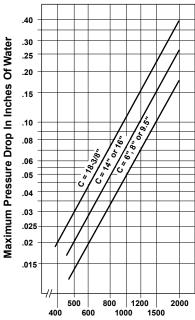
Chart A Velocity in SFPM Open Coil Design
