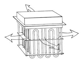
Vertically Mounted Tubular Or Finned Tubular Heater
