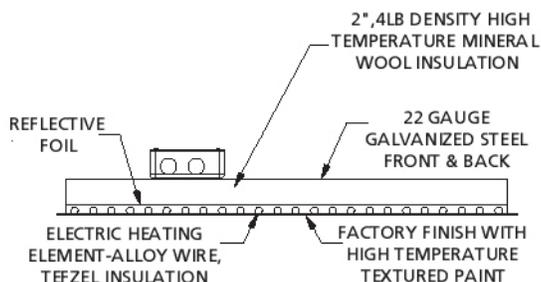
CUTAWAY VIEW OF SMARTROOMS
