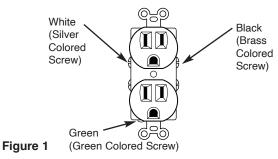
Use NEC Class 1 wiring system with wire suitable for at least 75°C. For receptacle use #14AWG copper.
